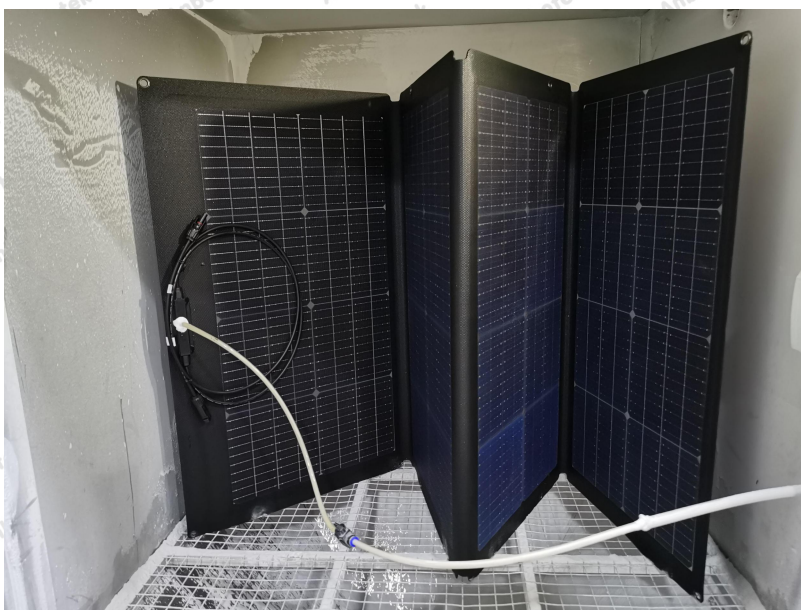
IP6X-Test set-up
